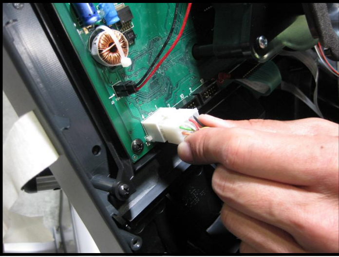
Step 5. Disconnect the 12-pin serial connector from the display
